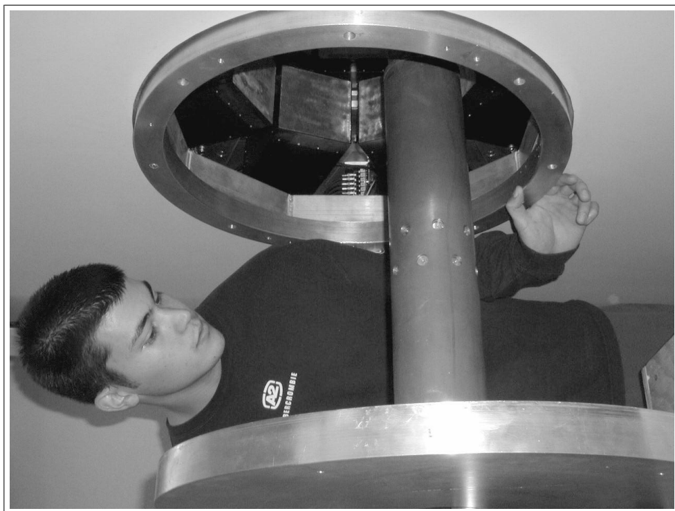
FIGURE 1.6. FastSPECT-II. On the left is a schematic image of FastSPECT-II, rendered from the original CAD design. The 16 cameras are solid, the housing and structure are wire-frame. On the right Lance Fesler shows the central lead pipe and gold pinhole collimators. Several modular cameras are visible inside the housing. (CAD by J. Butters, T. Lerdal, S. Lieber, and B. Stuckey. Photo by L. Furenlid.)
